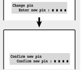
As soon as the 4 digits are entered, the "Confirm new pin" screen appears. Re-enter the same 4 digits. When the Confirm screen disappears, your PIN has been memorized. Press **MENU** three times to exit.
